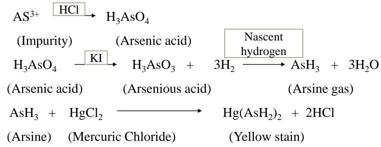
The depth of the yellow stain depending upon the amount of arsenic present in the sample is compared with that of standard stain produced from a known amount of arsenic.
